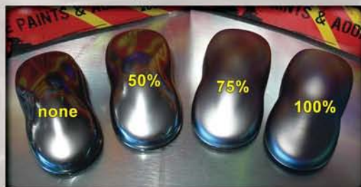
MirraChrome™ speedshape topcoated with varying amounts of Flattening Agent™
